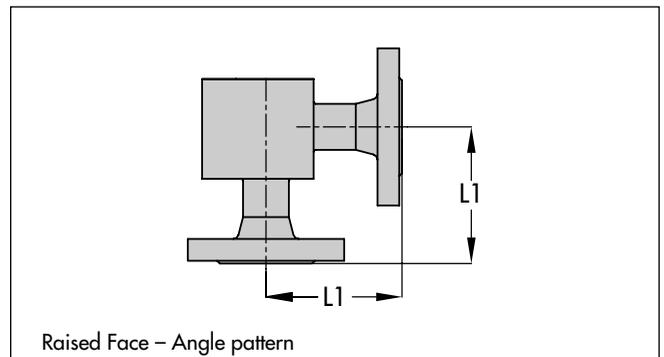
**Face-to-face and end-to-end dimensions for globe control valves according to ISA and IEC · Dimensions in inches**
